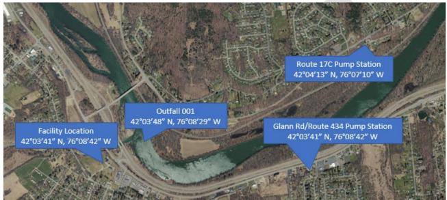
Type I Sanitary Sewer Overflows (SSOs) are classified as permanent emergency overflow structures which are designed, approved, constructed, and intended only for emergency discharges. Type I SSOs are typically located at or immediately upstream of a pump station or at the headworks of the treatment plant.
