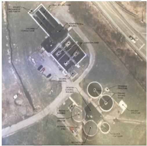
This is a publicly owned treatment works that receives flow from domestic users. Wastewater consists of treated sanitary. The sewage collection system consists of separate sewers. The treatment plant was constructed to provide secondary treatment for a design flow of 2.0 MGD.
