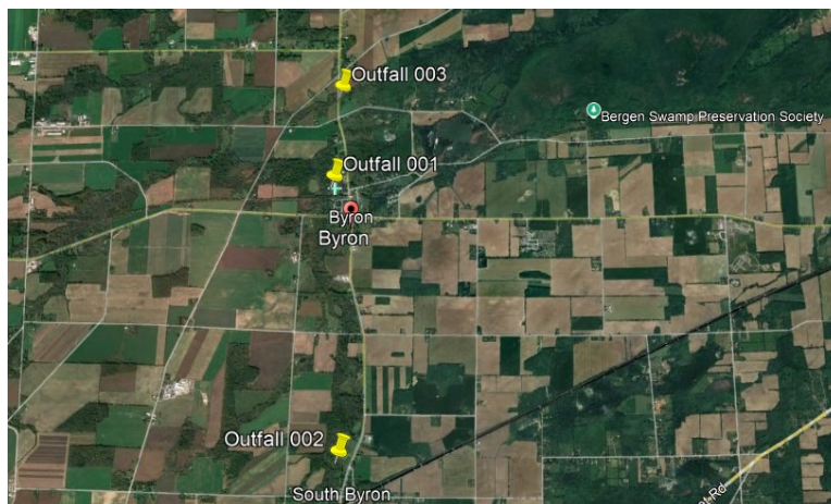
Figure 1: The Town of Byron WWTF consists of three physically separate facilities combined into one SPDES permit. Outfall 001 is near Central Byron, Outfall 002 is near South Byron, and Outfall 003 is near Pumpkin Hill on Spring Creek, which is a tributary of Black Creek. A new pump station will be constructed at South Byron (Outfall 002) to direct flows from South Byron to Central Byron. This will result in the consolidation of Outfall 001 and Outfall 002, reducing the Town's number of discharge points from three to two. Outfall 003 will remain the same and not be discussed further.
