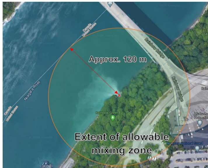
Figure 6: The image on the left shows a detail drawing of Outfall 001 from the permittee’s NY-2A Application. The image on the right shows the outfall and maximum extent of the mixing zone.
