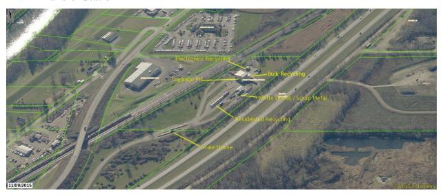
The Erwin Transfer Station is the largest of the Steuben County operated transfer stations, handling in excess of 9,000 ton per year mixed MSW and up to 1,000 ton per year Recyclables.
