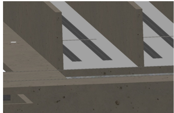
Photo 7 - Baseplate embedded in the bay floor
